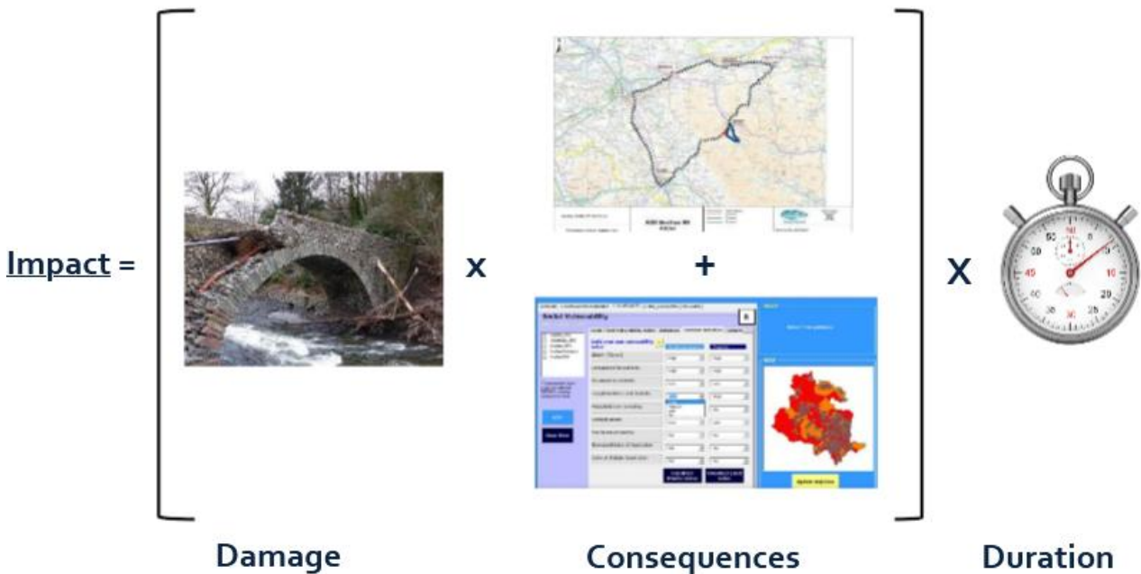
Figure 1 illustrates this formula in practice: physical damage to an asset assessed against the network consequences of that damage — including access to critical infrastructure, community connectivity, and vulnerability of the surrounding population. Source: UKRI/DfT-funded Network Resilience programme, DfT & LGTAG.
