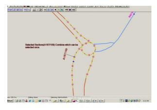
Figure 3.7 One section (A167/109) covers an area that should be 5 individual sections
