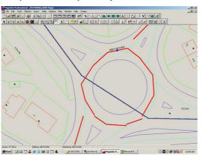
Figure 3.2 No connectivity (gaps before roundabout).
