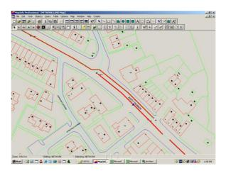
Figure 3.3 Section overlaps and no connectivity leaving a small unaccounted for section of road.
