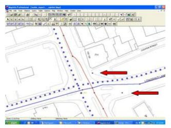
Figure 3.10 Missing dual carriageway section in network and section nodes (which are shown as small stars near the red arrows) are in incorrect positions.
