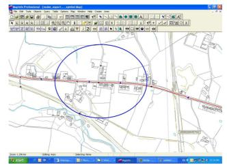
Figure 3.11 Directions of sections is incorrect. The sections on the left of the circle run to the east whilst the sections on the right of the circle run to the west.
