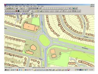
Figure 3.5 Inconsistent start/end locations resulting in the network length being longer than measured length (the sections start and end in the roundabout).
