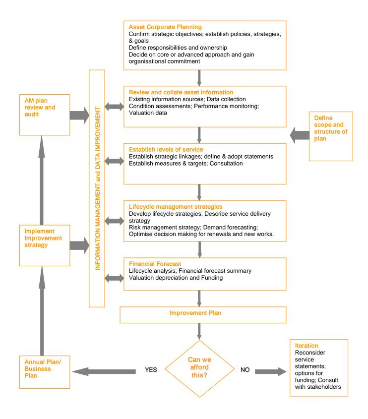
Figure 2 Roadmap for developing an asset management plan.
